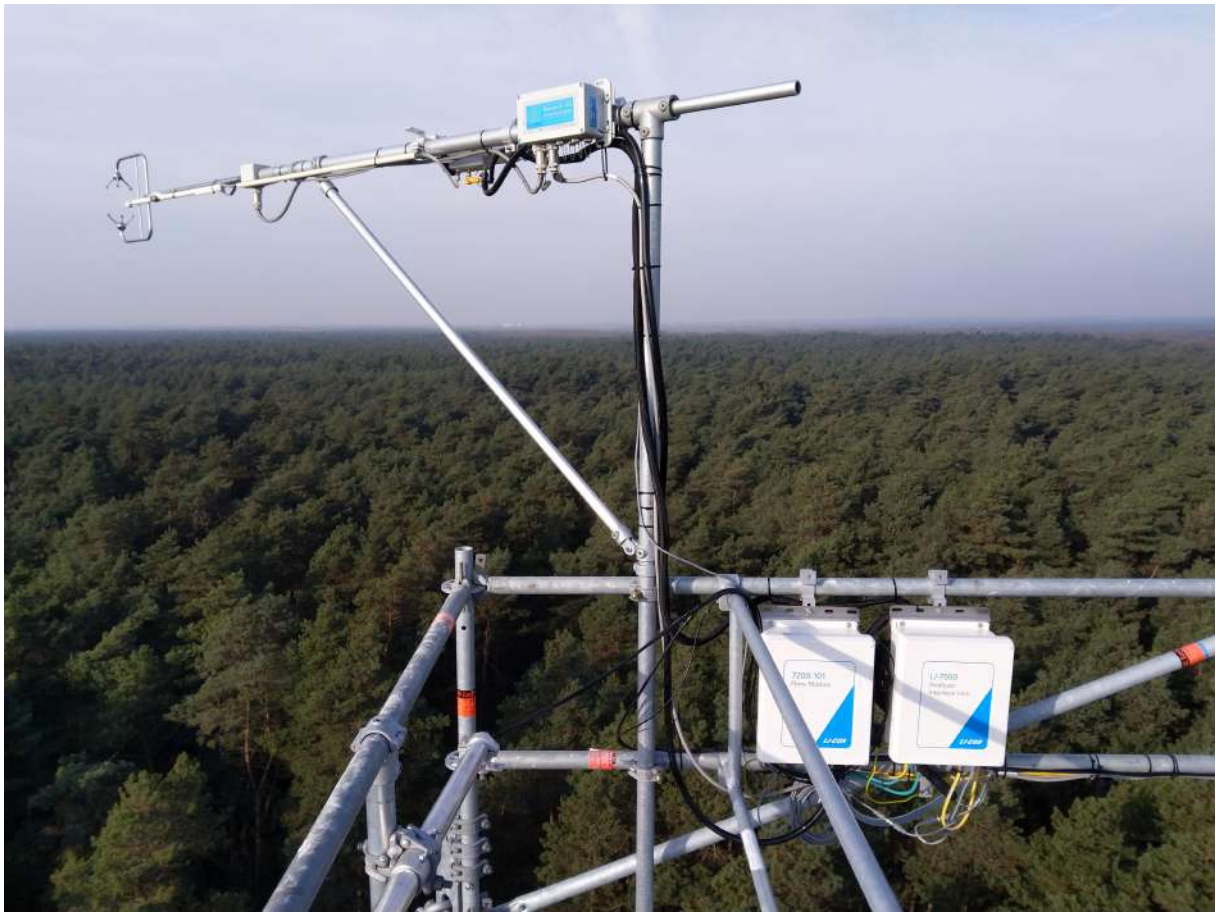
Photo 2: The eddy covariance system for fluxes of momentum, sensible and latent heat and CO 2 and VOC fluxes.
