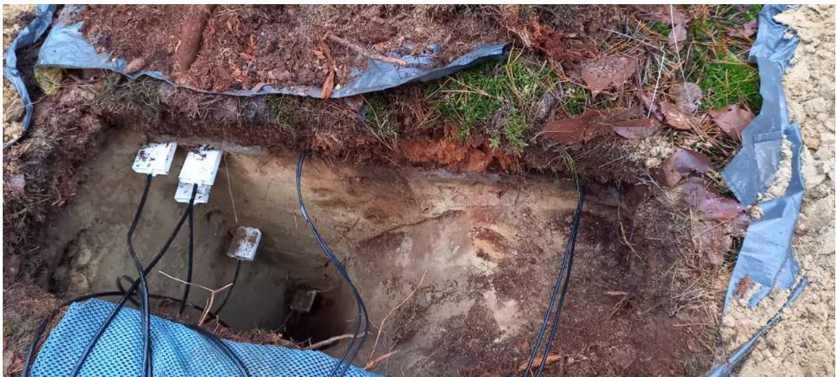
Photo 3: Soil pit for (left) soil temperature, soil water content profile, (middle) soil heat flux and (right) 2 more soil temperature sensors. This is one of the two extended locations. The other two locations do not have the deeper sensors.
