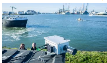
Figure 4. Since Nov 2018, KNMI measures tropospheric NO 2 with a MAXDOAS instrument in Rotterdam, at DCMR station Geulhaven. The measurements are performed every 5-15 minutes during daytime. They serve as a validation source for satellite measurements (e.g. TROPOMI), and regional air-quality models (e.g. CAMS, LOTOS-EUROS).
