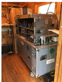
Figure 3. At one Rotterdam site RUG & WUR will perform Atmospheric O 2 measurements which provides additional information on CO 2 emissions from fossil fuel combustion, as the oxidative ratio (O 2 /CO 2 ratio) is different for each type of fuel. The oxidative ratio for the global average fossil fuel mix is around 1.4, whereas this ratio is much higher for natural gas (1.95). Atmospheric O 2 will therefore allow to attribute the emissions to specific source categories. The figures shows the instrumental set-up which is currently tested in Finland.
