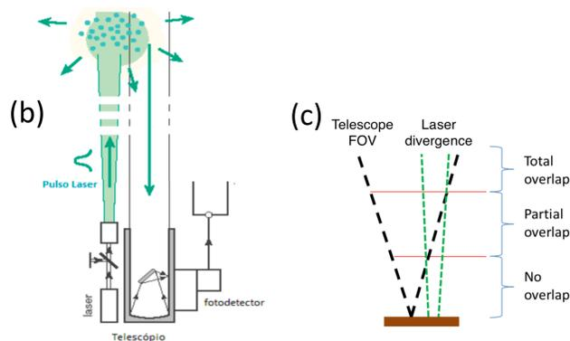
**Fig.1.** (a) The Raman lidar Caeli in operation at the Cabauw Experimental Site for Atmospheric Research (CESAR), close to the 213 m high meteorological tower. (b) Schematic of the Lidar remote sensing. (c) Overlap of the Lidar remote sensing.
