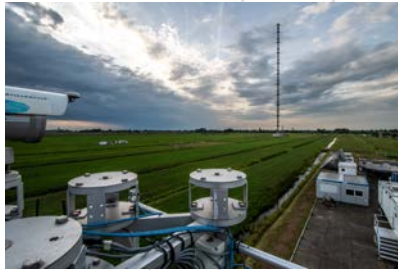
Scintillometer installed in Cabauw
