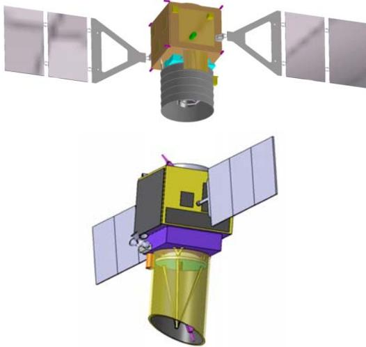
Figure 1: A-SCOPE spacecraft configuration with IPDA lidar concept at 2.05  $\mu\text{m}$  (top) and 1.57  $\mu\text{m}$  (bottom)
