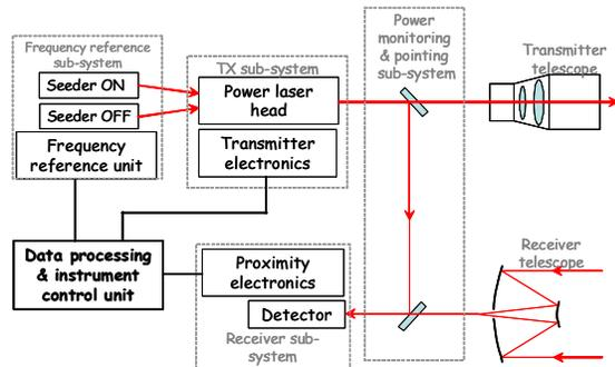
Figure 2: Functional block diagram of the IPDA instrument architecture
