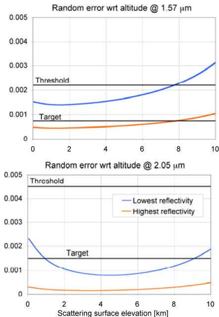
Figure 3: DAOD relative random error performance computed as a function of the ground elevation
