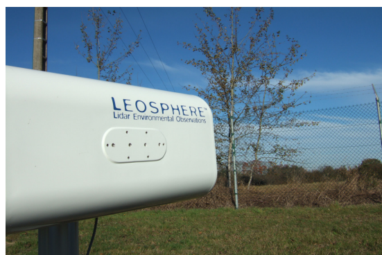
Figure 1: EZ Lidar™ ALS450 during the ICOS Campaign
