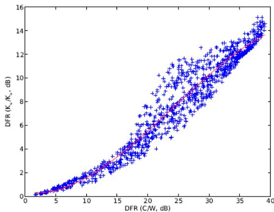
Figure 3. Simulation of dual frequency ratios in snowfall for Ku/Ka and C/W band radar observations.
