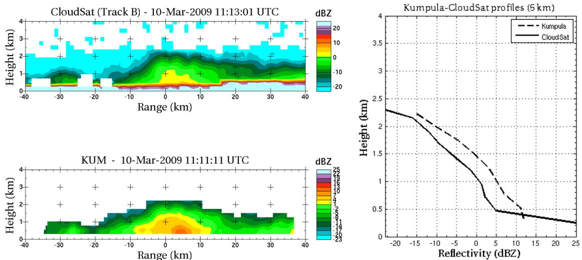
Figure 2. Simultaneous observations of precipitation that took place on March 10, 2009 by using CloudSat and University of Helsinki Kumpula radar.
