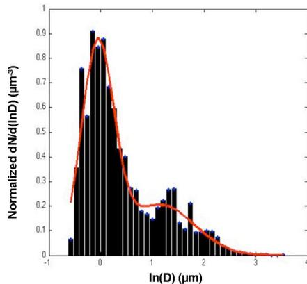
Figure 6. Normalized number size distribution of particles according to the logarithm of their Ferret diameter.
