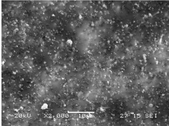
Figure 5. SEM image for  $PM_{2.5}$  filter collected on February 7, 2009.
