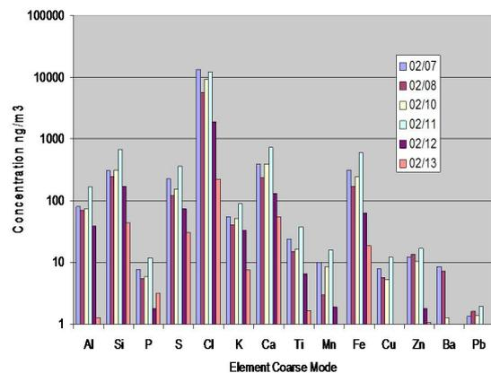
Figure 7. Elemental composition of fine and coarse particulate matter samples analyzed with PIXE.
