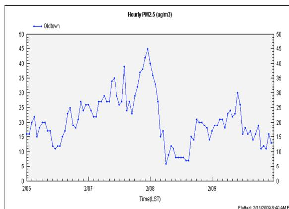
Figure 3. Hourly PM<sub>2.5</sub> concentrations recorded at Maryland Department of the Environment Oldtown Monitoring Station during the elastic lidar observations.
