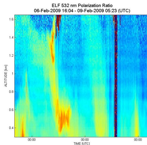
Figure 4. Elastic lidar polarization ratio timeseries for February 6-9, 2009. Particle scattering within boundary layer are due to non-spherical particles.
