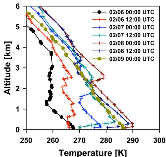
Figure 1. Temperature profiles from radiosonde launches at Dulles International Airport, Virginia during February 6-9, 2009. Profiles with cross symbols show temperature inversions below 850 m during pollution event.
