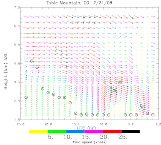
Figure 7. Hourly wind profiles produced by high-resolution WRF model at the TBM profiler location for 31 July.
