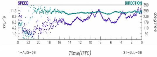
Figure 4. Wind speed and direction measurements from the Continental Divide meteorological station (CDE) at 2 m AGL for 31 July.
