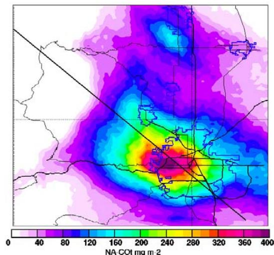
Figure 8a. Column concentration of CO derived from WRF-driven FLEXPART model in the Front Range area on 1 August, 00 UTC. Black line indicates location of vertical cross section shown in Figure 8b.
