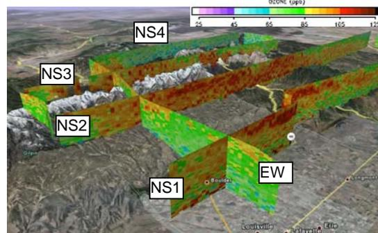
Figure 2. Vertical cross section of ozone measured with the TOPAZ lidar on 31 July, 21:30 – 1 August, 00:30 UTC. Data extend from near the surface to about 4.6 km ASL.
