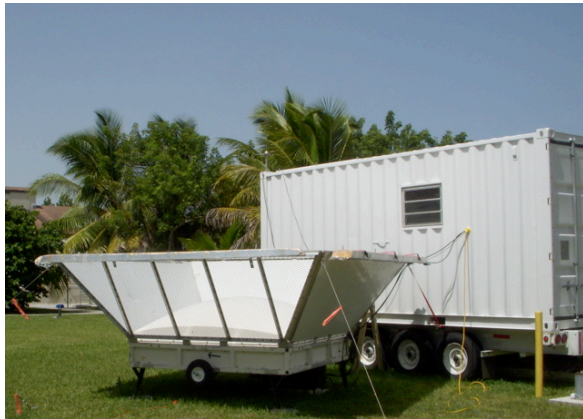
Figure 1: The NCAR MAPR wind profiler at CPS.
