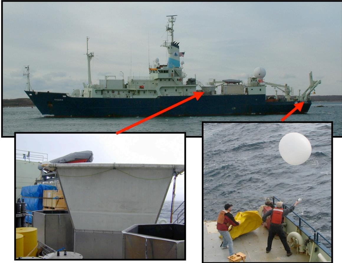
Figure 1: The R/V Knorr (upper photo), the wind profiler (lower left), and a radiosonde sounding (lower right).
