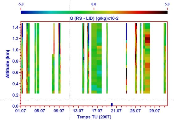
Figure 6. Time evolution of lidar humidity profiles during July 2007.
