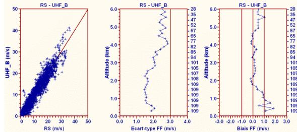
Figure 2. Statistical comparison of the horizontal wind data obtained from the UHF wind profiler (UHF) versus those measured by radio sonde (RS). Left: Scatterplot of wind values (x-axis RS measurements, y-axis UHF), Middle: Standard deviation with height, and Right: Bias with height. The numbers at the right of middle and right figures represent the number of cases taken for the statistics at each range.
