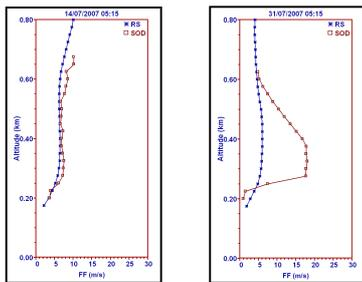
Figure 3. Some examples of comparison of wind speed between radio sounding (RS) and sodar (SOD)
