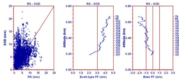
Figure 4. As in Fig. 2, but using sodar wind data versus those measured by RS
