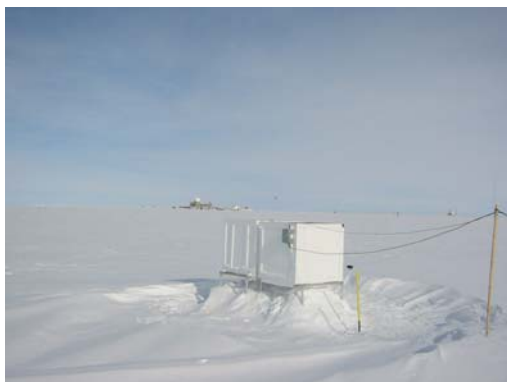
Figure 7. The bistatic sodar is shown with its separate transmit and receive systems (used to reduce the contamination produced by the ringing of the transducer).
