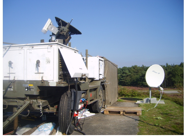
Figure 5. The bird radar “Superfledermaus” equipped with a camera mounted parallel to the radar antenna
