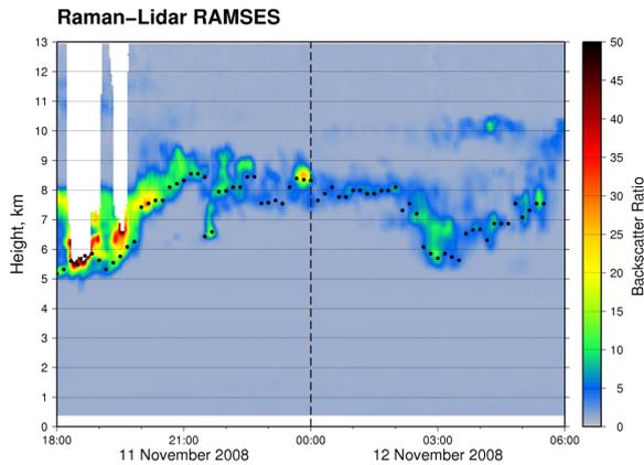
Figure 1: RAMSES - backscatter ratio in color shading. White areas indicate rejected low-quality data, the black dots indicate 10-minute averages of cloud base measurements from a ceilometer on site
