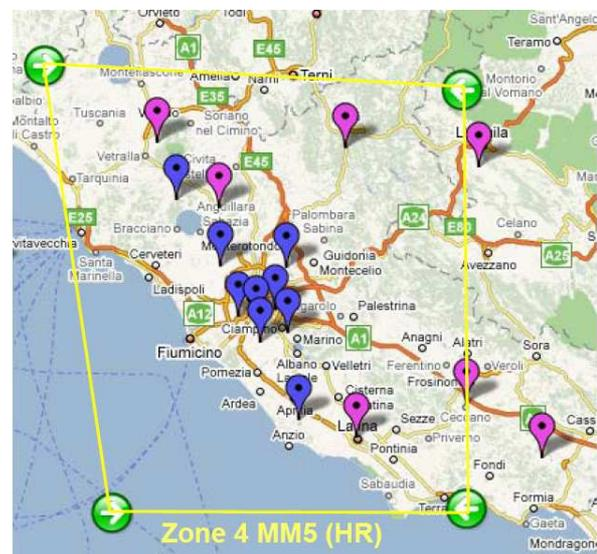
Figure 1. Frame of the MM5 higher resolution domain and location of the operational GPS network.
