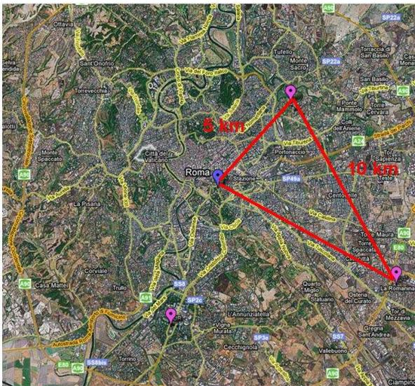
Figure 2. The network of microwave radiometers. The MWR is located on the DIESAP anchor site (marked in blue) while the 3 CMR are located on the vertices of the red triangle. Radiosondes were launched from DIESAP.
