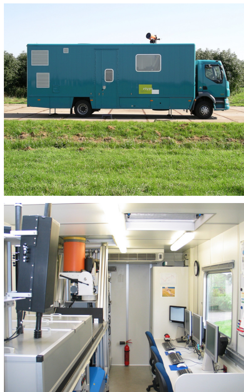
Figure 1. The mobile lidar, exterior and interior.
