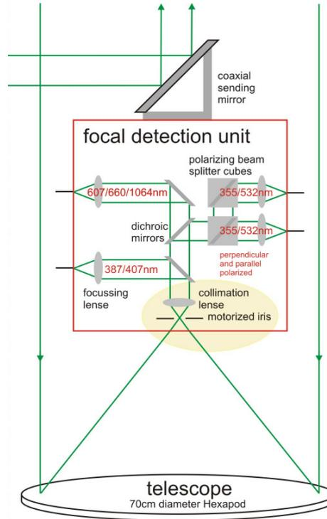
Fig.2: The focal detection unit
