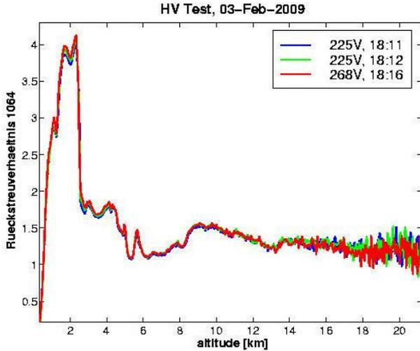
Fig.3: The backscatter in IR does not depend on the APD volatage
