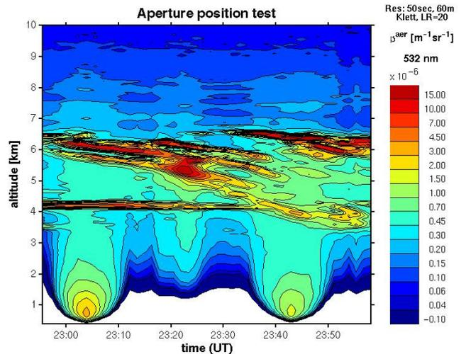
Fig.5: Tests with moving aperture from 1mm (infinity focus) to 5mm (focus at 615m).
