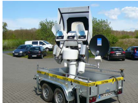
Figure 7. ADMIRARI instrument: Three frequency (10.7 / 21.0 / 36.5 GHz), dual polarized radiometer, optimized for rain observations.
