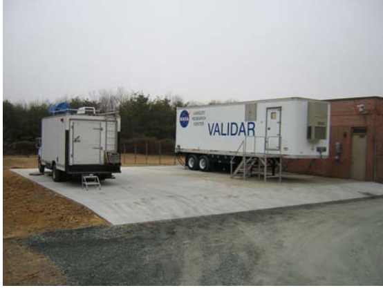
Figure 1: Photograph of field test site at the Howard University Research Campus in Beltsville, MD. The lidar is housed within a 35-foot long trailer testbed called VALIDAR. The other trailer houses the Godard Lidar Observatory for Wind (GLOW).
