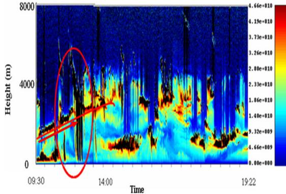
FIGURE 1. Range-corrected signals at 1064 nm wavelength throughout the measurement period on 20 July 2007.
