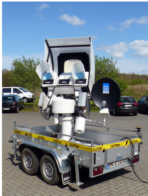
Figure 5. ADMIRARI three-frequency dual polarization radiometer at RPG facilities. The fully steerable radiometer is mounted on a trailer. A Micro Rain Radar is attached to the scanning mechanics.
