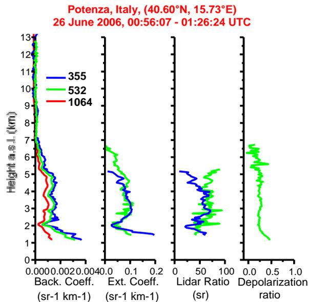
Figure 1. Saharan dust outbreak occurred over the Mediterranean basin measured over Potenza on 26 June 2006. Shown are profiles of the particle backscatter coefficients (blue = 355nm, green = 532 nm, red = 1064), the extinction coefficients, the lidar ratios and the linear depolarization ratio.
