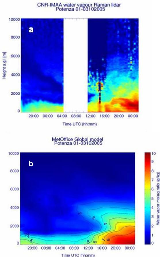
Figure 4. Comparison of the time series of the vertical profile of the water vapour mixing ratio as measured by the CNR-IMAA water vapor Raman lidar (a) and as retrieved by the MetOffice Global model (b) on the period from 1 October at 16:25 UTC to 3 October 2005 at 01:34 UTC
