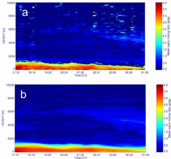
Figure 2. Time series of the water vapor mixing ratio profile as measured by the water vapor Raman lidar operational at the CNR-IMAA on the 26-27/02/2006 (a); time series of the water vapor mixing ratio profile obtained using the integration algorithm based on the Kalman filtering algorithm (b).
