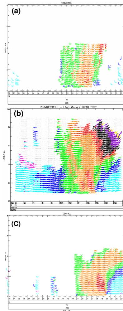
Figure 11. Wind barb plots of wind speed and direction from (a) Cobba-combe Doppler weather radar winds and (b) Dunkeswell 1290 MHz wind profiler radar (c) Clee Hill Doppler weather radar on 3<sup>rd</sup> March 2009.
