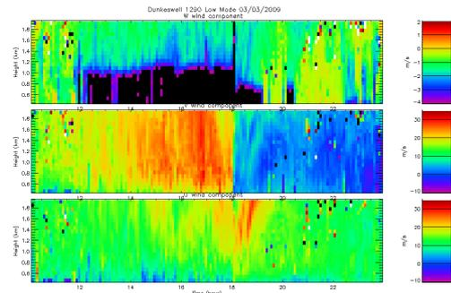
Figure 8. Analysis of the W (top), V (middle) and U (bottom) wind components from the Dunkeswell 1290 MHz operated in low mode profiling radar on 3<sup>rd</sup> March 2009.
