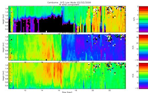
Figure 5. Analysis of the W (top), V (middle) and U (bottom) wind components from the Camborne 915 MHz profiling radar operated in low mode on 3<sup>rd</sup> March 2009.
