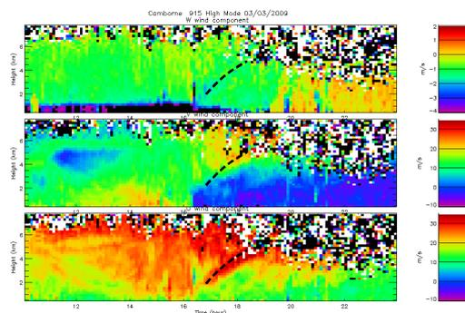
Figure 4. Analysis of the W (top), V (middle) and U (bottom) wind components from the Camborne 915 MHz profiling radar on 3<sup>rd</sup> March 2009.
