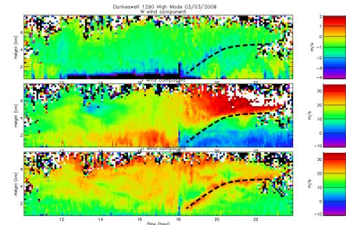
Figure 7. Analysis of the W (top), V (middle) and U (bottom) wind components from the Dunkeswell 1290 MHz profiling radar on 3<sup>rd</sup> March 2009.
