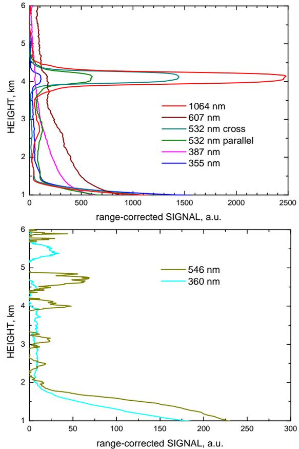
Figure 3. Range corrected signals. Top: regular MWL signals measured at March 31, 2009 from 10:30 to 11:30 UTC. Bottom: Raman quartz signals at 360 and 546 nm measured with MWL at March 31, 2009 from 14:27 to 17:27 UTC.
