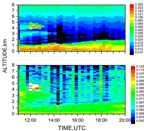
Figure 2. Time series of the observation of March 31, 2009 over Gwangju, Korea. The top panel shows the extinction coefficient in  $\text{km}^{-1}$ . The bottom panel indicates the linear volume depolarization ratio. The data have been obtained with the depolarization lidar of KOPRI.
