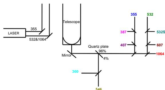
Figure 1. Schematic of the GIST Multi-wavelengths Raman lidar.
