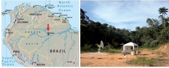
Figure 1. Left: Map of northern South America. The red arrow shows the location of the field site for the lidar observations. Right: Field site with the satellite dish for internet connection and the lidar Polly XT .
