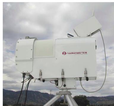
Figure 2. Profiling radiometer TP/WVP-3000.
