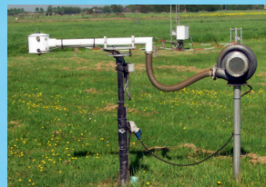
Figure 2. Eppley radiometers, measuring longwave upward and downward radiation.
