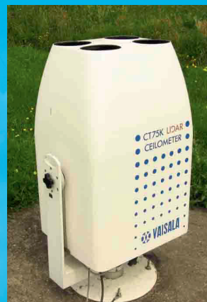
Cloud Lidars LD 40 and CT75K (shown), detecting cloud base height.
