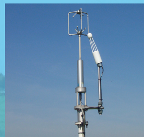
Figure 3. Sonic anemometer Gill R3 and Licor 7500 open path H 2 O sensor.
