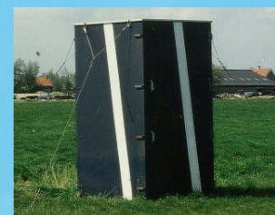
Figure 3. The mixing height is monitored by a monostatic acoustic sounder from Aerovironment.
