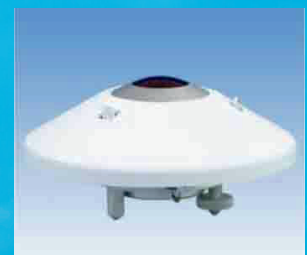
Pyreometer, observing global downward radiation, fed into an algorithm to estimate cloud cover.
