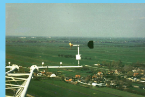
Figure 1. Gill propeller vane 8002DX to measure wind speed and direction.
