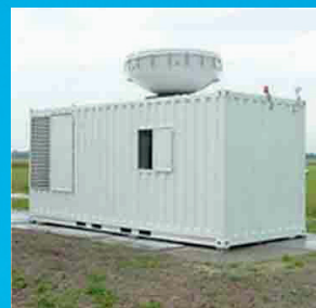
Cloud Radar (35 GHz), used in combination with the Lidar.
