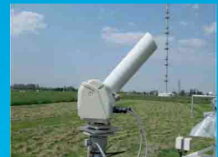
NubiScope, an infrared pyrometer, scanning the whole hemisphere.
