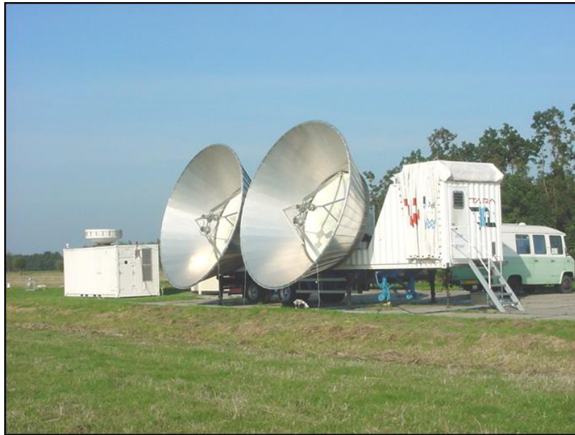
Figure 1: TARA (right) at the remote sensing site at Cabauw next to the KNMI 35GHz vertically pointing cloud radar (left).
