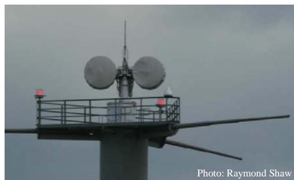
Figure 1: IDRA on top of the Cabauw tower. IDRA uses two antennas, one for transmit and one for receive.
